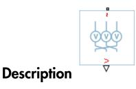
The Line Voltage Sensor block represents an ideal three-phase line voltage sensor. The block measures the line-line voltages of a three-phase system and outputs a threeelement physical signal vector. Each element of the physical signal output vector is proportional to the voltage between the phases as follows:
